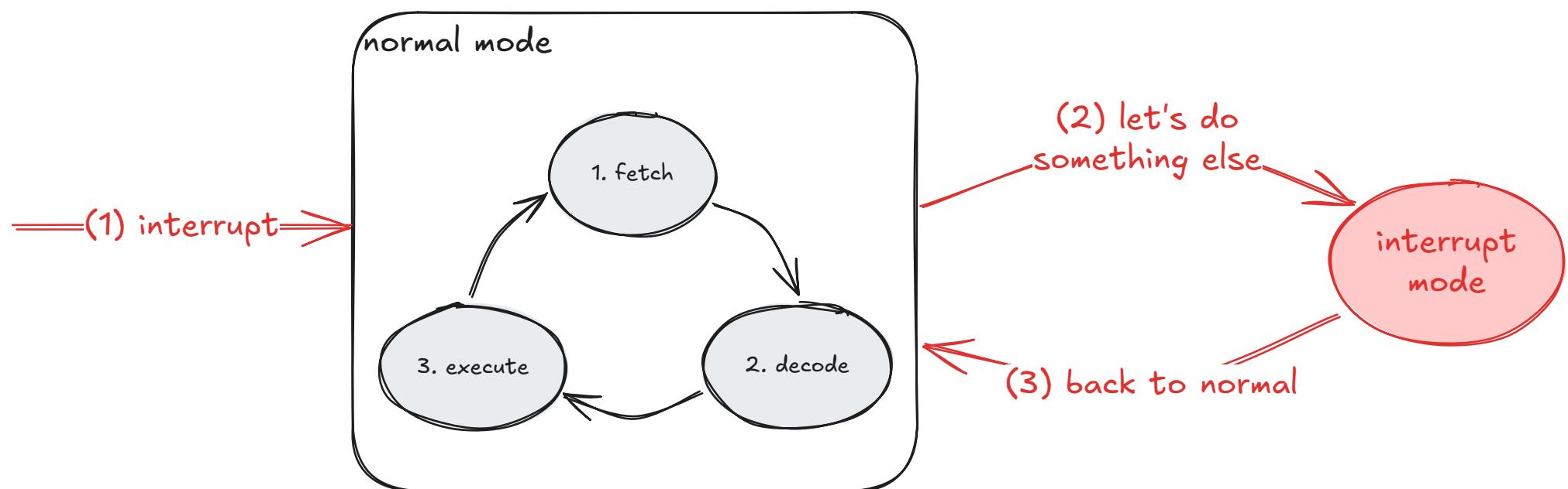
Each CPU has an Interrupt Controller attached which triggers the mode switch
