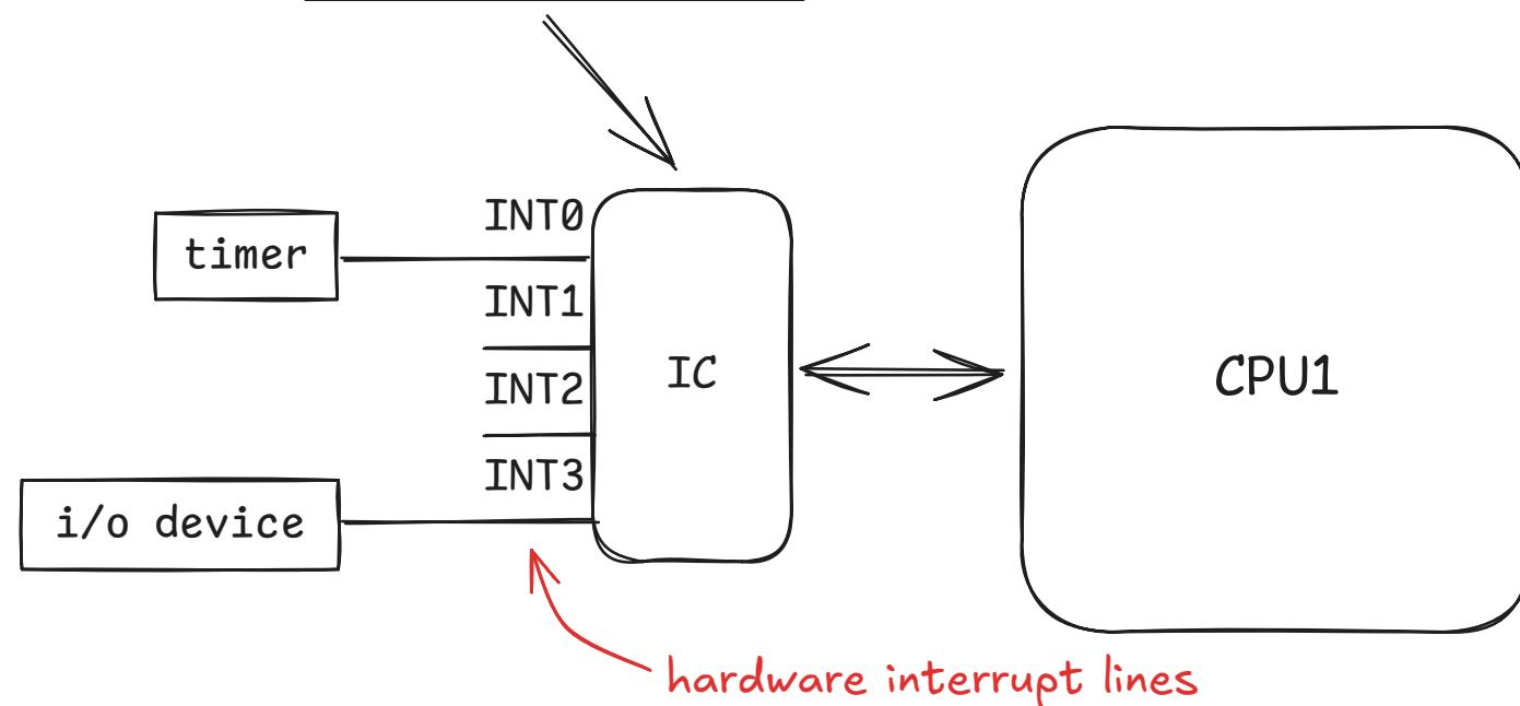
OS code configures the timer to fire an interrupt in a few milliseconds with a special instruction before jumping to the user code.
