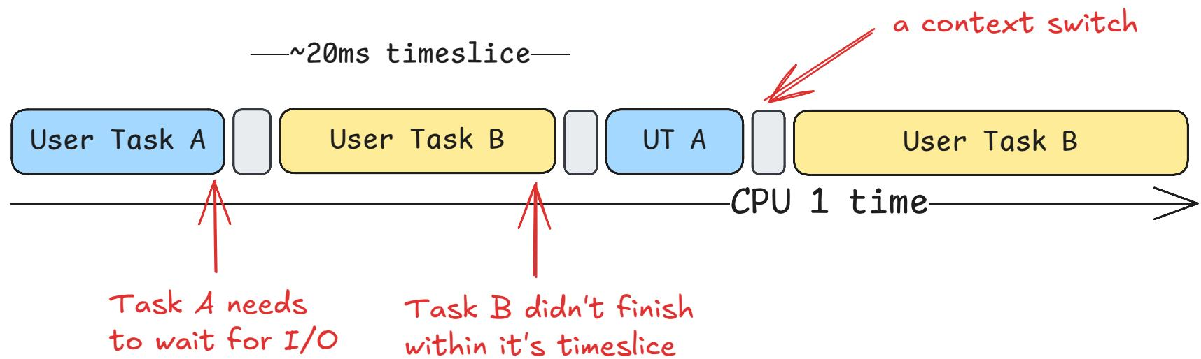
The OS must be able to take the CPU from a running task and assign it to some other task
