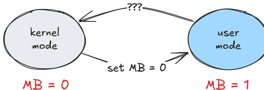
A single bit stored within the CPU core, set to 1 when running the OS code.
