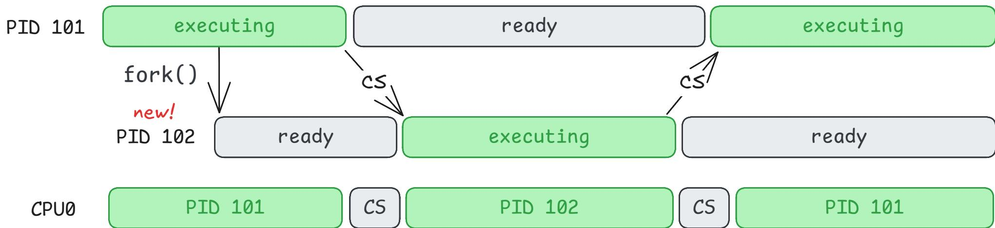
During fork() handling system allocates and initializes a new PCB along with necessary resources. This new PCB is then yield to the scheduler as a new ready queue element.
