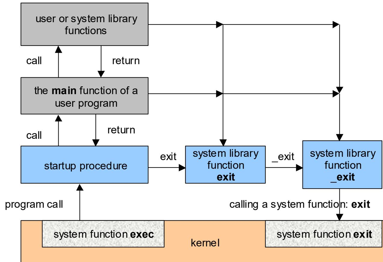
From process creation (system function **exec**) till process termination (system function **exit**)
